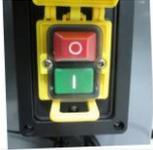
To start the machine, press the green button "I".
