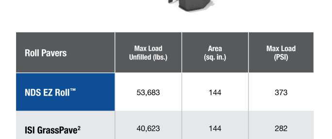
NDS Max load for soil-filled cells is 400,000 lbs.
