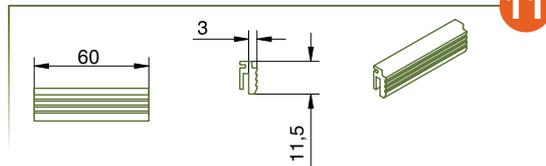
**5** Joint de guidage autocollant DK0.419\*\*\*
