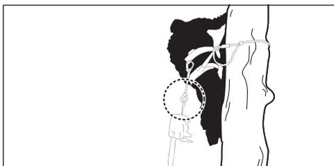
When moving the product from any one attachment point to another, the operator should ensure that it is secured in the new position before releasing it from the previous attachment point.
