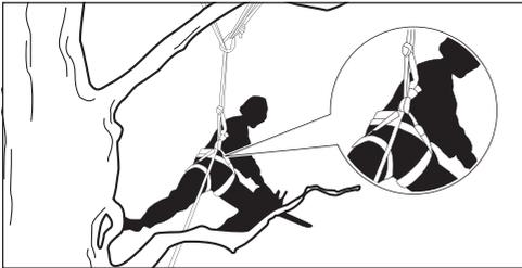
Gaining a secure footing at the work position can be aided by the use of a temporary foot stirrup created from an endless sling.
