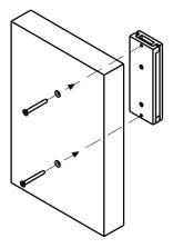
1.) Door Knocker can also be mounted bolt-through. Drill in with a distance of 130mm two holes with ø 5,5 mm through the door Pay attention that you drill rightangled to the door leaf.
