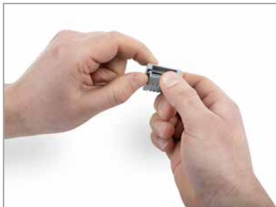
Open the Gelbox with the side latch.
