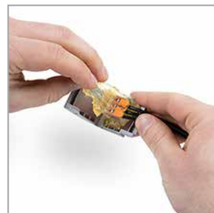
Easy circuit extension: Open the Gelbox, remove the gel from the connector, open the connector and connect the new components to the cable.
