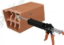
Feed the hole from the end to the external surface by going back from 1 mixer graduation between each pump.
