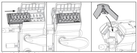
Step 6: Replacing the closing cover.
