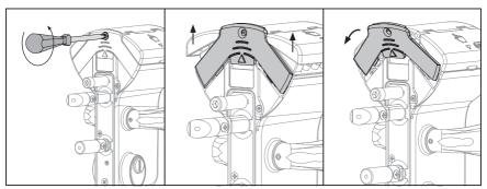
Step 2: Slide both code panels out of the lockbox.
